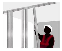
For heights that exceed the maximum manufacturer stud length, the Hadley I Studs would require to be spliced as per our recommended splicing detail. DRY-HAD-XX-ZZ-DT-X-1912
